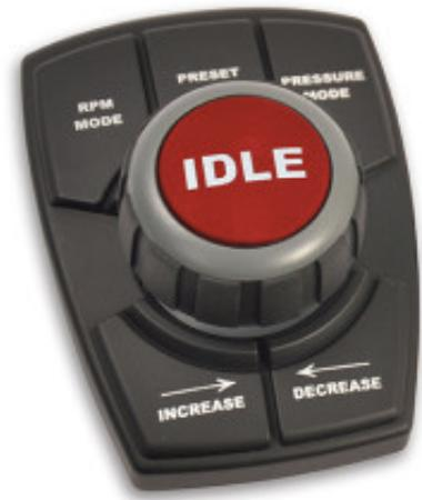
The Matrix Pressure Governor monitors and controls your pump discharge pressure to maintain desired operating pressure range. With intelligent controls, it detects conditions when water supply is reduced or cut off and reacts the way an operator would to keep engine speed from increasing out of control.
