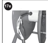
Connect the Black, White and Green wires from your cord set to the three matching colored wires exiting the cord reel's center hub.(Red if a 4 wire reel is purchased.) Hand crimp each connection with heavy duty wire crimps designed for crimping. Make sure that there are no loose wires or wire strands around the butt connectors.
