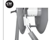
Slide the shrink tube down your cord set wire and over the three butt connectors to the reel hub.
