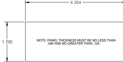
REQUIRED PANEL CUTOUT DIMENSIONS FOR SNAP-IN MOUNTING
