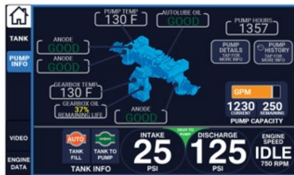
Figure 18. Pump Flow And Reserve Pump Capacity
