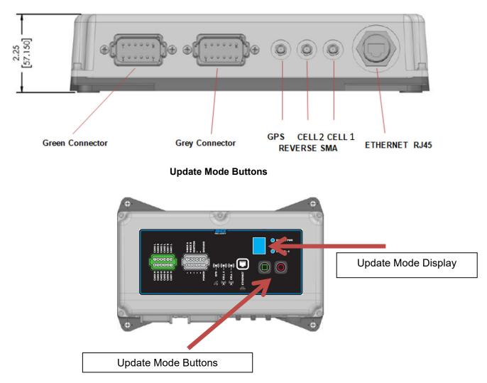
Telemetry Control Unit Device hardware can accept an Over-The-Air update to both the Telemetry Control Unit Device hardware device OS as well as accept remote multiplex updates for both V-MUX and ES-Key systems. The Telemetry Control Unit Device hardware device must be physically placed into program accept mode to allow a remote user to send a file down to the box. To do this, users must:
