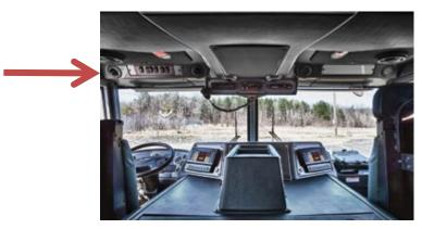
• In the vehicle example shown above the preferred areas were not suitable for mounting the Telemetry Control Unit Device hardware. As an alternative, we were able to mount the Telemetry Control Unit box on the rear of the engine cover inside the cab and us a support brace to get the antenna cabling up to the roof.
