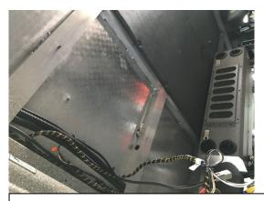
Headliner removed – Note Harness and potential cross member interference
