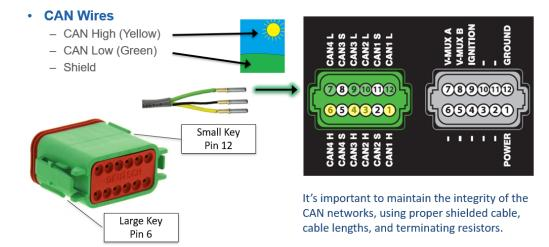
The shield wire should be pinned for all CAN port connections. The shield wire should NOT be pinned for the V-Mux connection.
