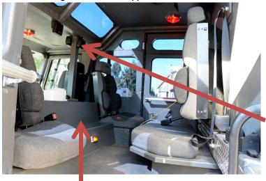
• While this is not the optimal location, our test vehicle had other electronics mounted in the same area with a protective cover over them. There was also a wiring chase that led to the center dash that allowed for power, ground, and communication bus wiring.
