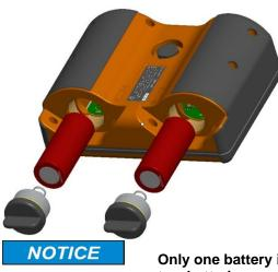
Only one battery is required to power the Wireless Remote Controller. If two batteries are installed, the battery with the highest voltage will provide power.
