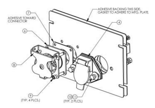
Figure 5 – 0N10-1037-00 Module Face Plate Sub-Assembly, Back side
