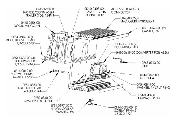
Figure 3 – 0N10-1038-00 Rear Module Sub-Assembly w/ Trialer Connector and Converter Module
