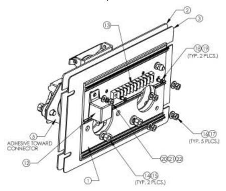
Figure 4 – 0N10-1037-00 Module Face Plate Sub-Assembly, Back side
