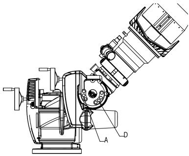
10. Set soft stops inside of the range of travel limited by the hard stop bolts.
