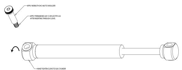
3. Assemble the gas spring to the monitor (1) as illustrated in Figure 5 below. Loosely assemble the mounting block, washers, and bolts (2) to the monitor. Apply Permabond LM113 or Loctite 222 to the threads.
